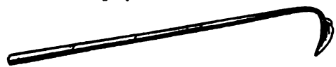
No. 2.—Length of handle, including iron socket, 4½ feet; handle of deal, and 1 inch diameter. The handle is marked in feet and inches. Length of blade, 4½ inches; breadth round, from edge to edge, 2 inches.
